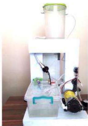
8) System simulation using a set of plastic containers, rubber tubes, valves with small 12v DC water pump with AC-DC adapter.
