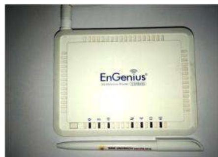
7) EnGenius 3G Wireless Router ESR6650. Represents the AP used to establish the wireless connection between the two microcontrollers.
