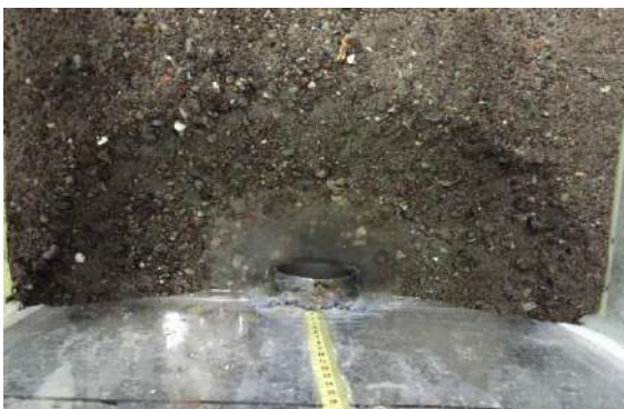
Top view of flushing cone (Photo 3)
