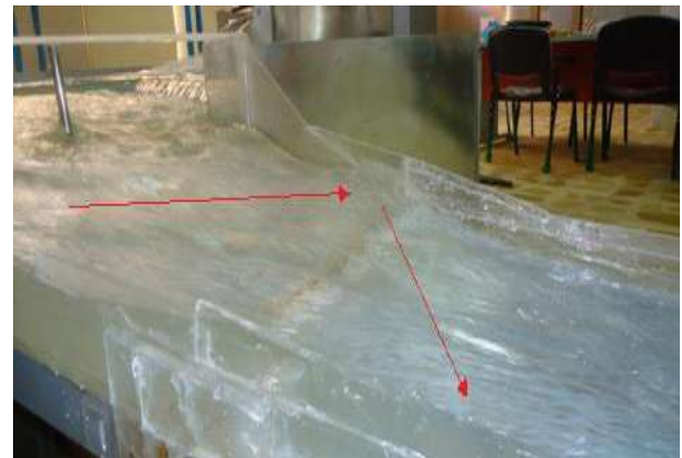
Figure 5 Cross waves in the transition and rising water level at side wall.
