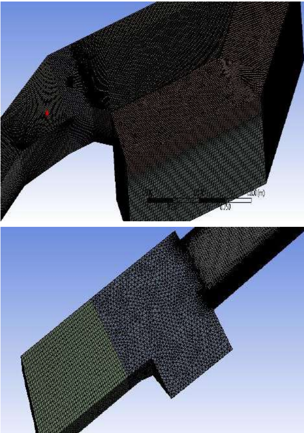
Figure 1 typical view of mesh generation for different parts of side channel spillway.
