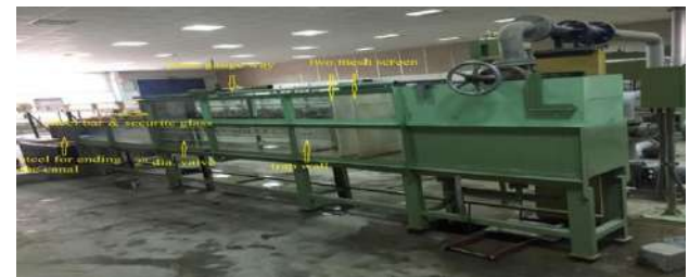
The flume and Main reservoir. (Photo 1)
