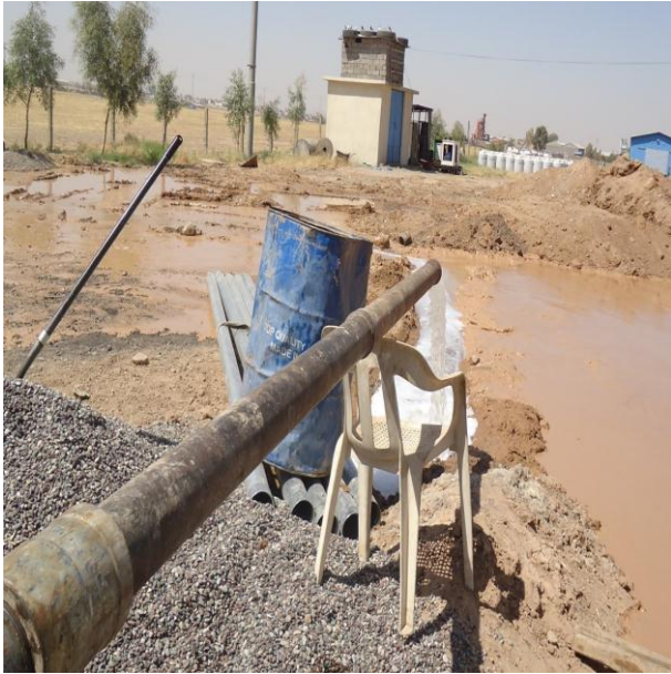
Figure 2 measuring discharge during pumping test
