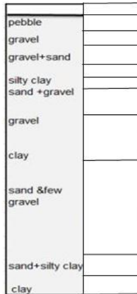
Figure 2: Geological profile taken from borehole test.
