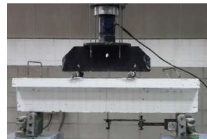
Figure 4: T-Beam geometrical detail with loading
