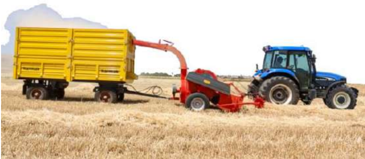
Figure 1. Tractor, straw picking up and chopping machine, and trolley.
