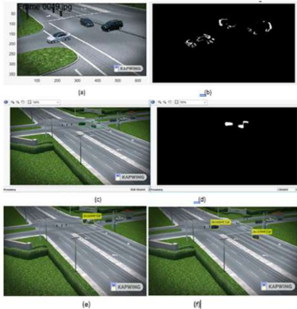
Figure 6: The original frame number 49 from carAccVideoOne (b) binary image of frame number 49 (c) detecting the car object from carAccVideoTwo (d) foreground segmentation of image frame number 254. (e) consider the vehicles as accidents cars for reporting. (f) label the vehicles that are close to making accidents.
