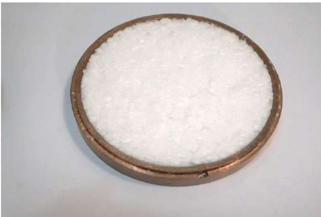
Figure (4) module sample 6mm filled with paraffin
