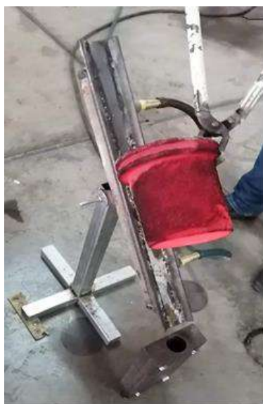
Figure (1): The cooling slope device.
