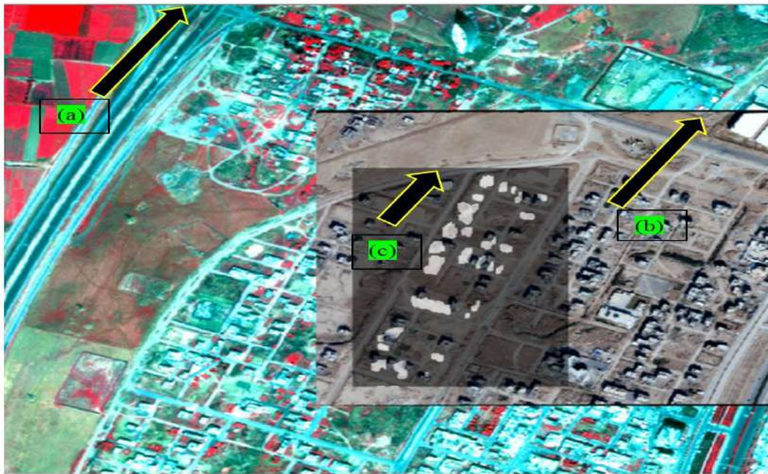
Figure (9) (a) satellite image, (b) ortho image generated from Aerial images, (c) binary change map layer. All layers are overlaid using arc map software
