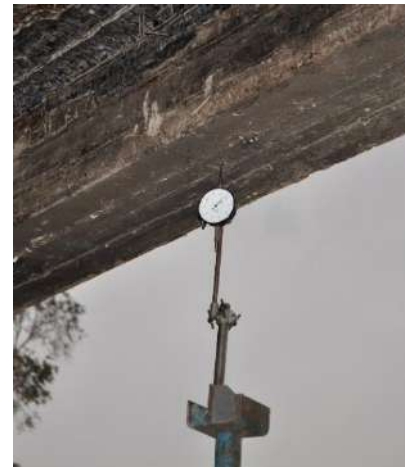
Figure 14: Installation of dial gage by using the magnetic base
