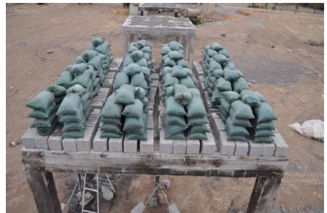
Figure 14: Applying full load by using sandbags
