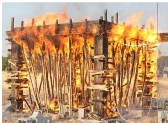
Figure 4: Reinforced concrete frame exposed to fire
