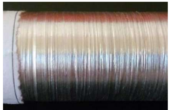
Figure 8: Deteriorated surface (higher than 100 \mu\text{m} ) produced by a tool of IA= 60^\circ , ECEA = 50^\circ and r = 0.5 \text{ mm} .
