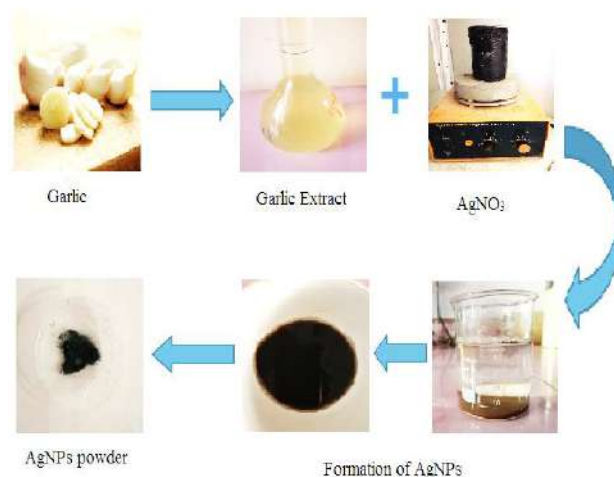
Figure (1): Synthesis steps of silver nanoparticle by green method.
