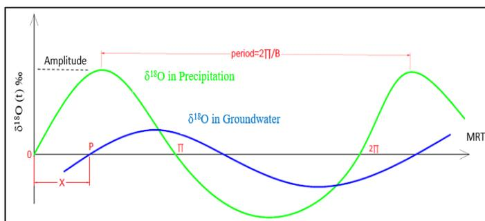
Fig. 2 Variation of  $\delta^{18}O$  in groundwater compared to the sinusoidal input from precipitation.
