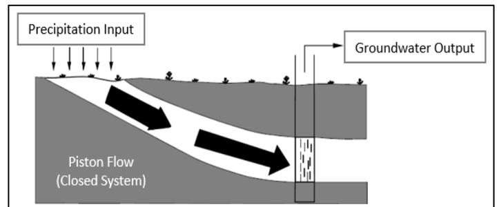
Fig. 1 Piston flow for groundwater movement (Texas Department of Transportation 2016).
