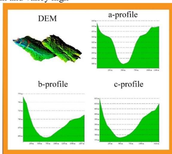
Figure 9: Three section profile locate by DEM Map a-profile section Bastora River on dam axis, b-profile section up stream on Bstora basin and c-profile section on downstream located on River.
