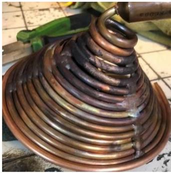
Figure 4: conical cavity receiver
