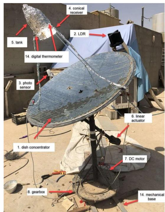
Figure 1: Solar thermal concentrator prototype
