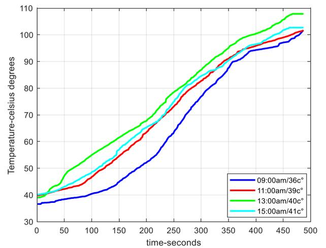
Figure 15: Tank rising temperature using the dual axis tracking system
