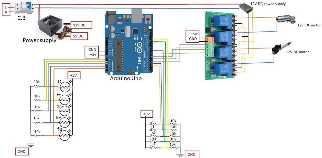
Figure 6: Dual axis tracking wiring diagram
