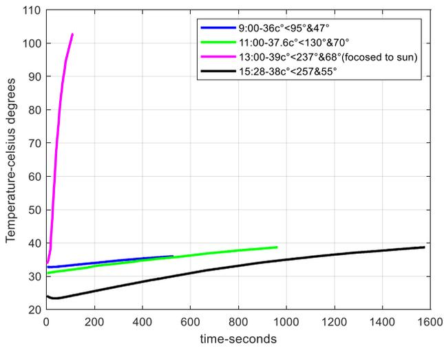
Figure 11: Receiver rising temperature without a tracking system.
