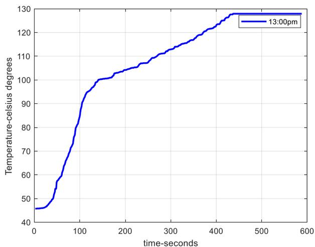
Figure 13: Water temperature inside conical cavity receiver
