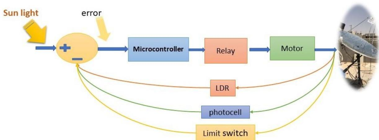
Figure 5: Block diagram of dual axis tracking system
