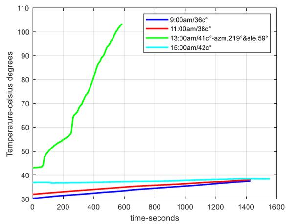
Figure 14: Tank temperature rising without a tracking system.
