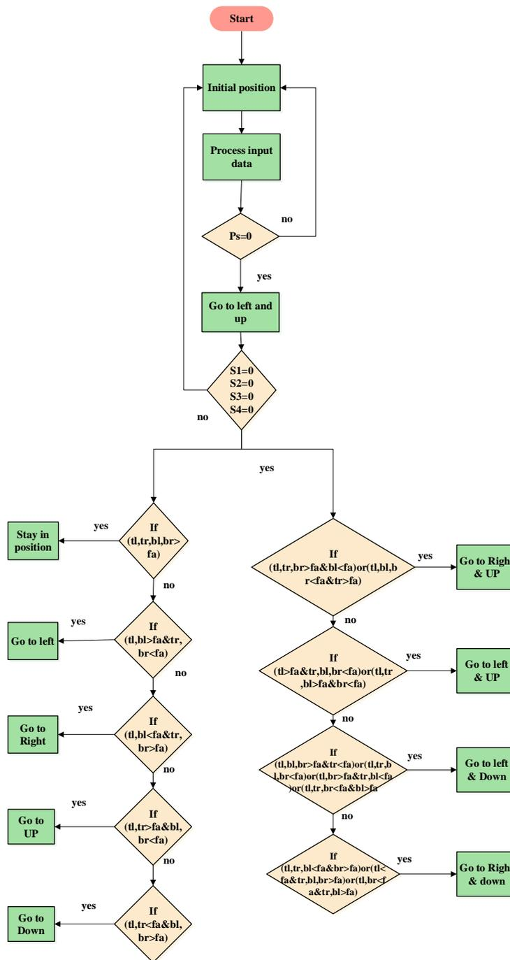
Figure 10: Flowchart of the dual axis tracking system controller
