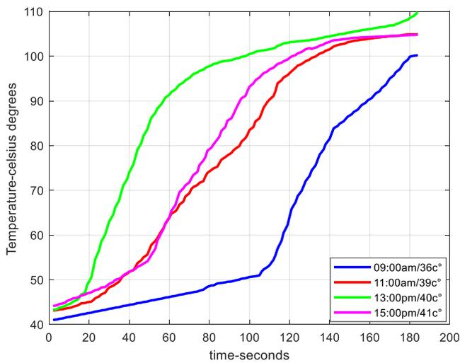
Figure 12: Receiver temperatures with the tracking system
