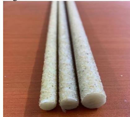
Fig. 1 Surface texture of the used sand-coated GFRP bars
