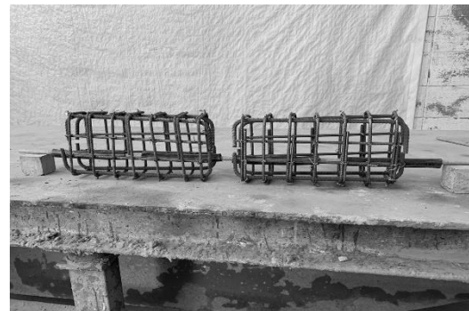
Fig. 2 Steel reinforcement of the beam specimens. The properties of the used materials concrete, sand-coated GFRP, and steel are represented in Table 1. The average cylindrical compressive strength of 21MPa is used as it was determined by using 150*300mm cylinders which is somehow equal to 25MPa with cubic compressive strength.
