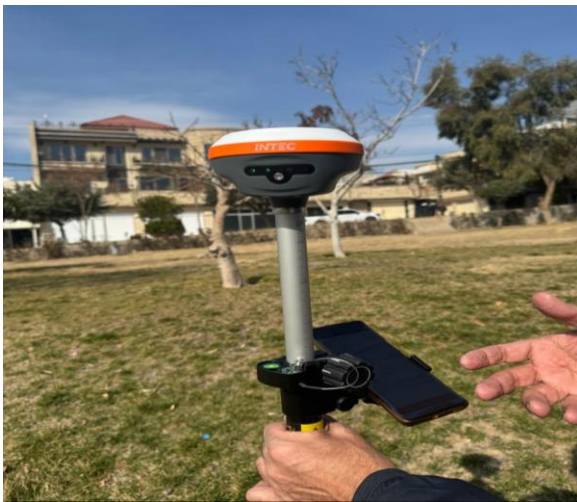
Figure 2: The Marvel laser GNSS receiver (INTEC)
