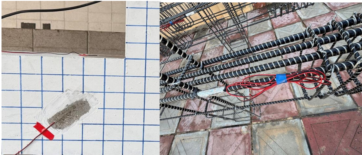
Figure 2. a) 50mm concrete strain gage, b) 3mm BFRP strain gauge
