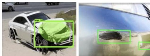
Figure 6. Mask RCCN car damage detection (COCO dataset)
