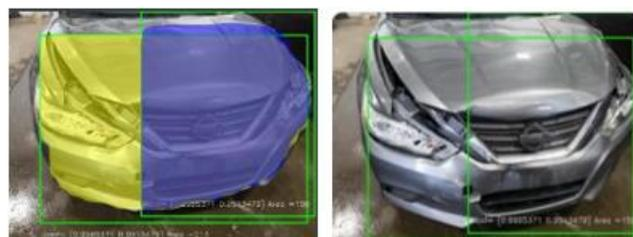
Figure 7. Mask RCCN car damage detection (Copart dataset)
