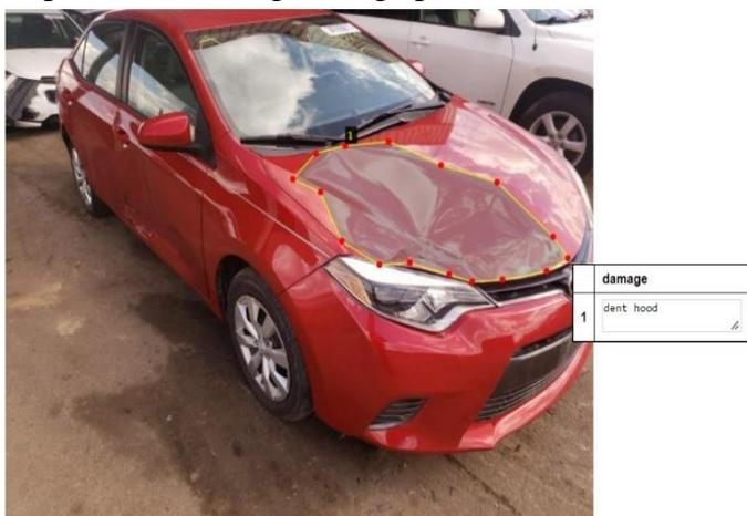
Figure 5. VIA labeled car-damage image
