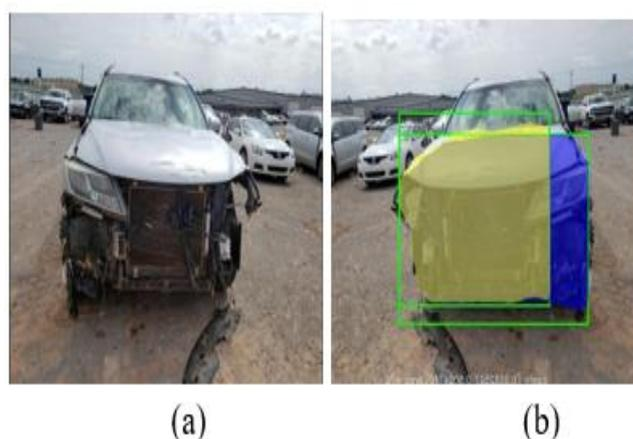
Figure 9. Damage localization. (a)Original front crash image, (b) The result of Mask RCNN (green box). Note that our proposed approach is capable to find the size and localize the area of the damage correctly.
