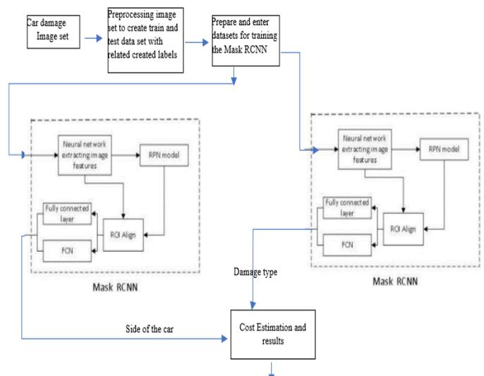
Figure 1: Detection of Car-damage and cost system framework
