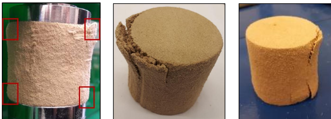
Fig. 5: Miscanthus test specimen during (left) and after the pressure test (middle, right)
