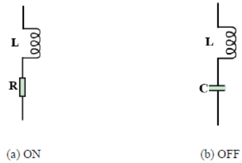
Figure 4. The equivalent circuits of the ON and OFF states.
