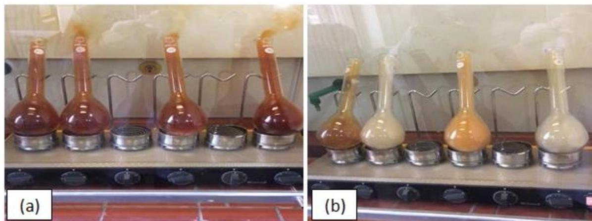
**Figure (1):** Wet digestion of the clay samples; (a) liberating brown fumes after addition concentrated  $\text{HNO}_3$ , (b) liberating white fumes after addition concentrated  $\text{HClO}_4$
