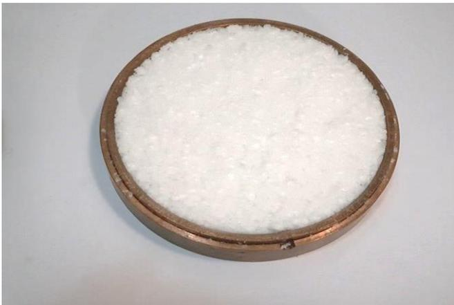
Figure (4) module sample 6mm filled with paraffin
