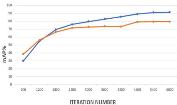
Figure 3: mAP of YOLOv4 and YOLOv4-tiny in the training process
