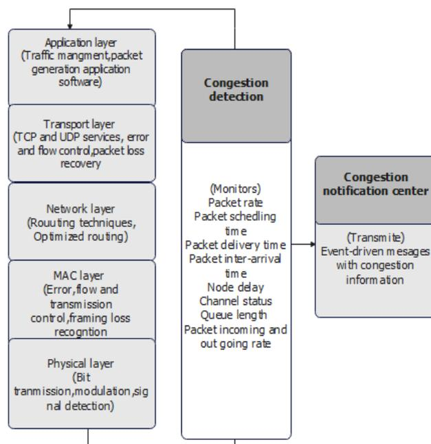
**Figure 5:** Cross-layer Procedure in Congestion Detection model.
