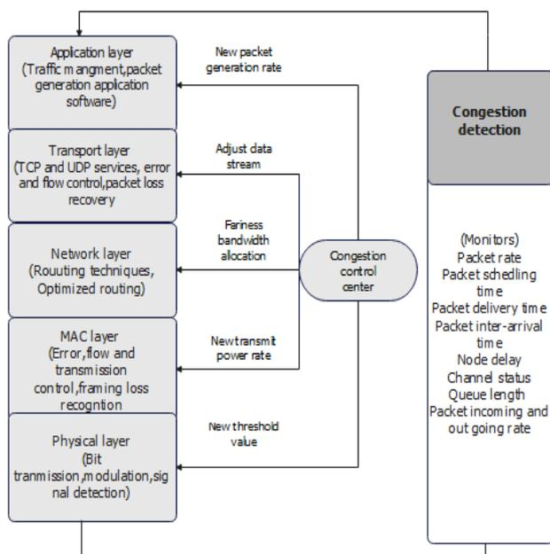
Figure 7: Cross-layer Procedure in congestion control.
