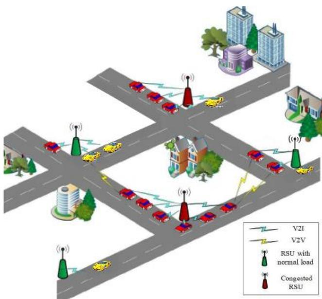
Figure 3: VANET Network (V2V, V2I)
