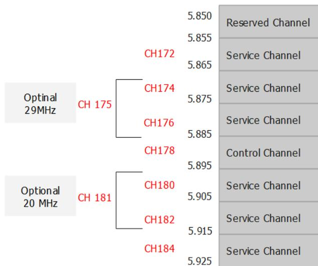
**Figure 1:** DSRC communication channel
