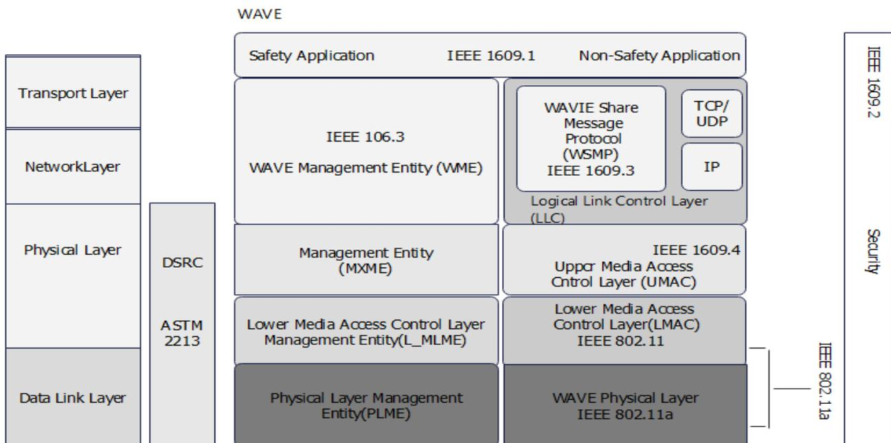
Figure 2: WAVE, IEEE-1609, IEEE-802.11p With Network Layers.
