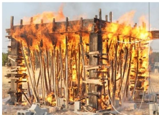
Figure 4: Reinforced concrete frame exposed to fire
