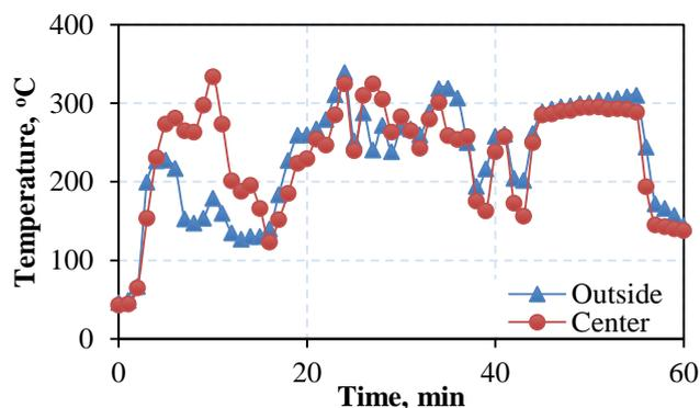
Figure 8: Time-temperature relationship of column at bottom
