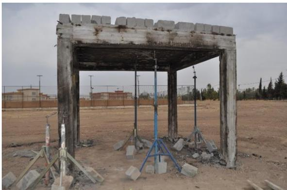
Figure 13: Location of installed dial gauges
