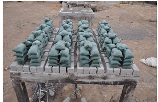
**Figure 14:** Applying full load by using sandbags
