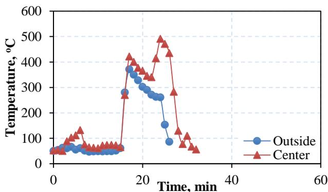
Figure 9: Time-temperature relationship of column at mid height
