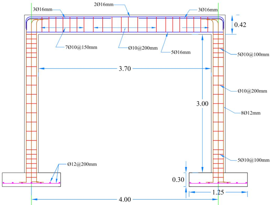
**Figure 2:** Reinforcement details of column, beam and footing
