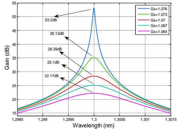
**Figure 5:** VCISOAs gain spectra in Reflection mode with different value of  $G_s$  and fixed  $R_b=99.9\%$  and  $R_f=86.6\%$ .
