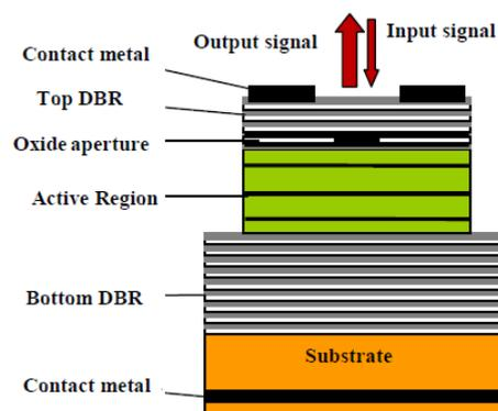
**Figure 1:** Typical VCSCOA structures of top emitting mesa. To make a VCSCOA amplifying, it requires mirrors with less reflectivity typically less than 99 % using DBRs.
