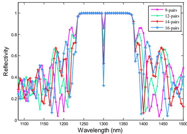
**Figure 3:** Reflectivity spectra for a cavity GaInNAsSb/GaAs VCISOAs placed between varied periods of front DBRs and 25-periods of back DBRs.
