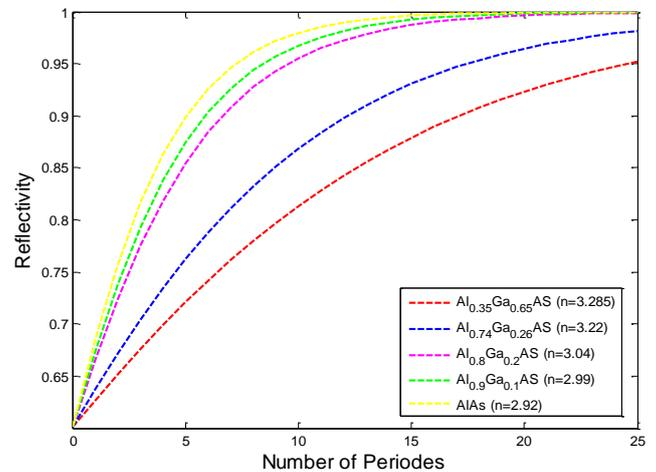
**Figure 2:** Distributed Bragg reflectors versus number of periods for different concentration of Al.
