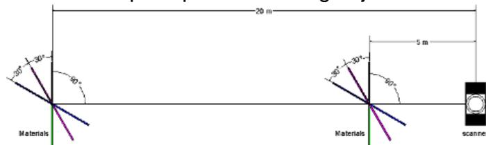
**Figure 4:** principal of Scanning materials using Faro focus premium TLS in 5m and 20m range and three different incident angles.
