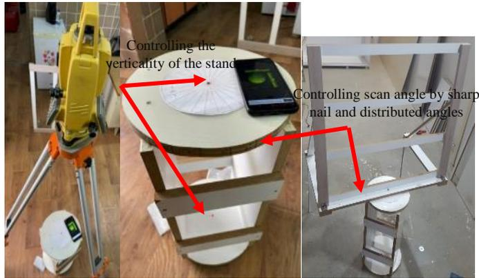
**Figure 3:** Verify the verticality of the stand by using the centering vertical laser beam of the total station equipment. The verticality test is shown by the two images on the right, while the controlling scan angle is shown in the left image.
