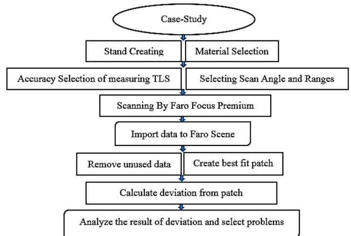
**Figure 2:** Flowchart illustrates the procedure of scanning and analyzing data
