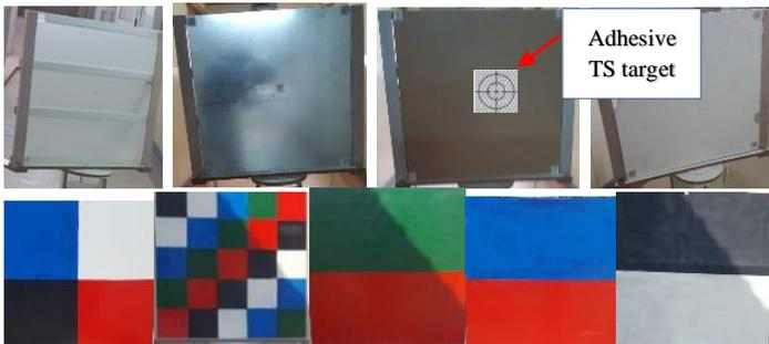
**Figure 1:** All materials performed for different angles of scanning and ranges using faro focus premium instruments, materials from left to right first row are: Glass, Steel, Wood, and Ekoplast, and second row are: painted materials from smooth to rough materials Alicobon, Gypsumboard, and Asropol
