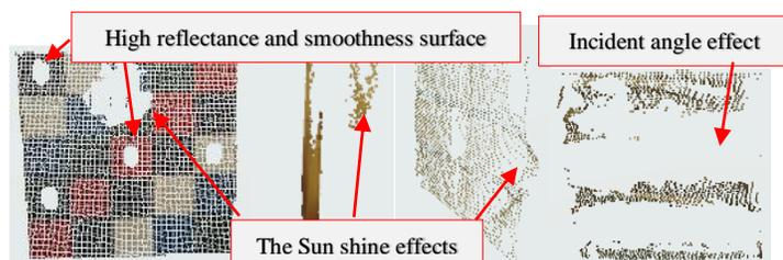
**Figure 10:** Errors happened on the smooth surface materials due to the Sun shine, incident angle and high reflectivity and smoothness of the materials.
