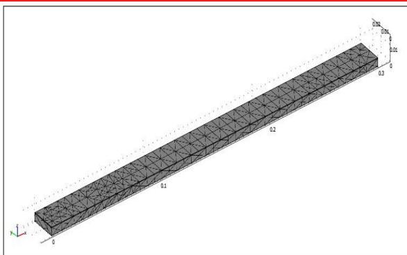
**Figure 2.a** The finite element model of a beam in COMSOL multiphysics software
