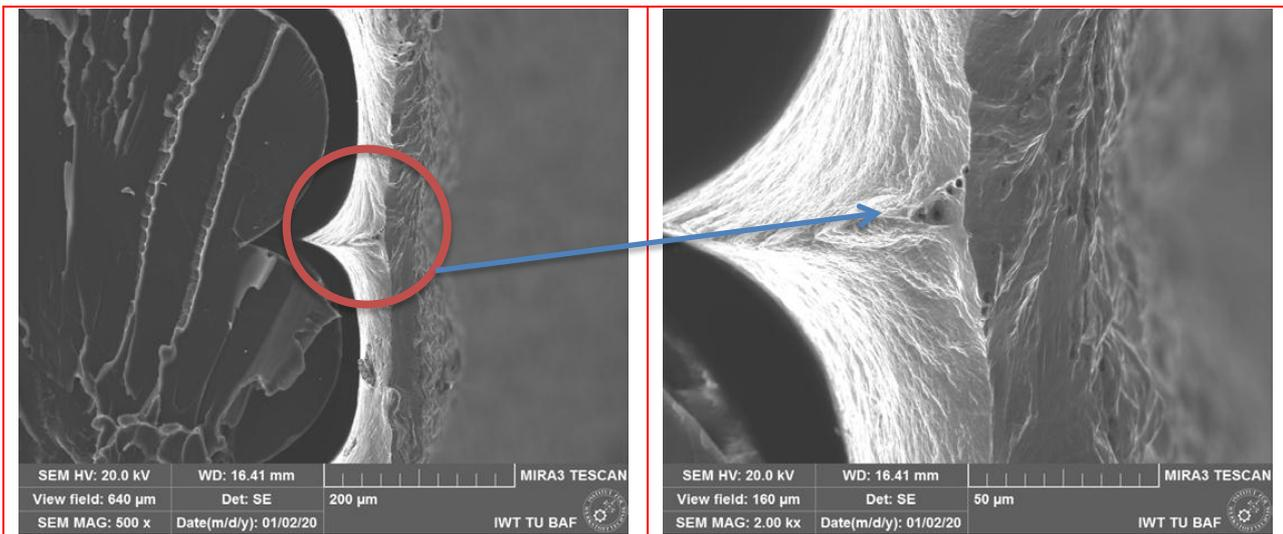
**Figure 8-a.** SEM image of the ULTEM 1010 coated with 100 µm Cu and 2 µm Ni.
