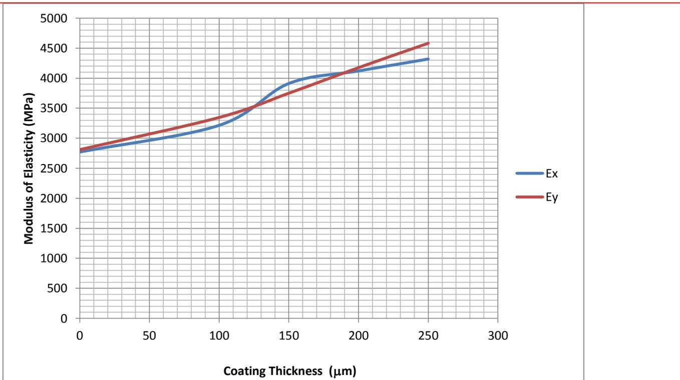
**Figure 7.** Modulus of elasticity for samples with different coating thickness made in x and y-direction
