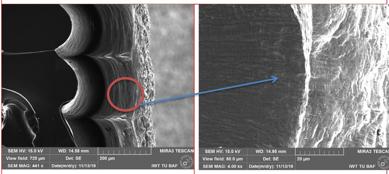
**Figure 8-d.** SEM image of the ULTEM 1010 coated with 250  $\mu\text{m}$  Cu and 2  $\mu\text{m}$  Ni.
