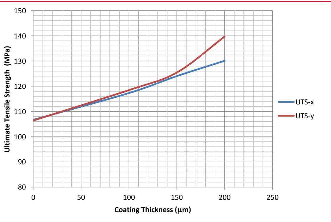
**Figure 6.** Ultimate tensile strength of samples with different coating thickness made in x and y-direction
