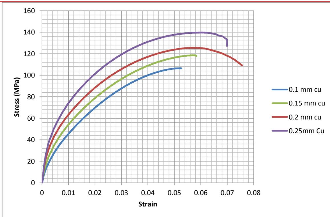
**Figure 5.** Strain-stress diagram for coated samples made in the x-direction.
