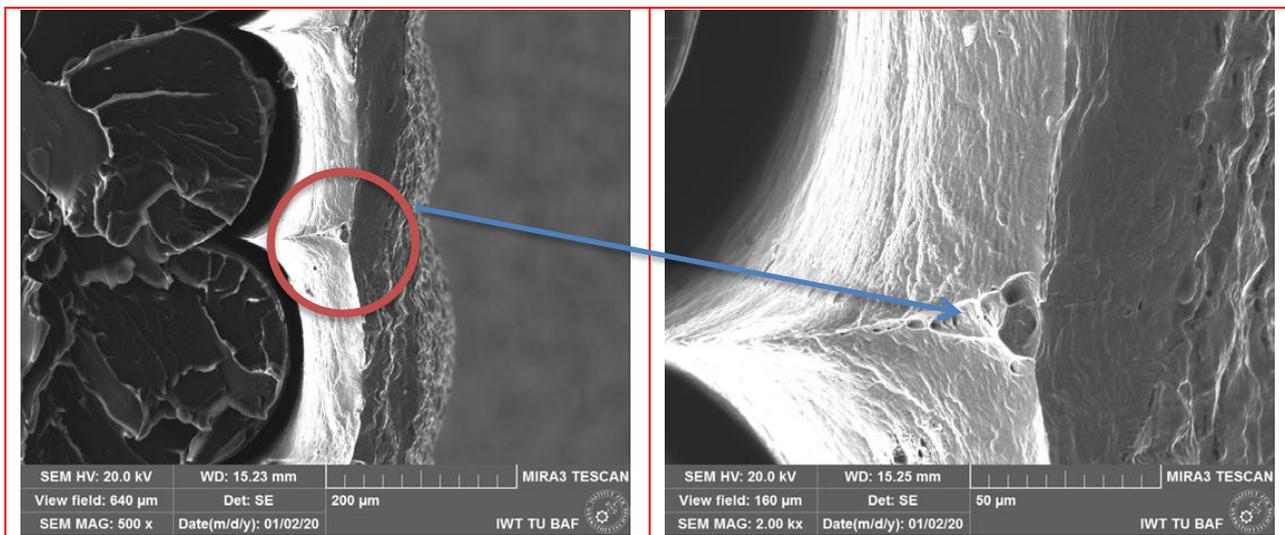
**Figure 8-b.** SEM image of the ULTEM 1010 coated with 150 μm Cu and 2 μm Ni.
