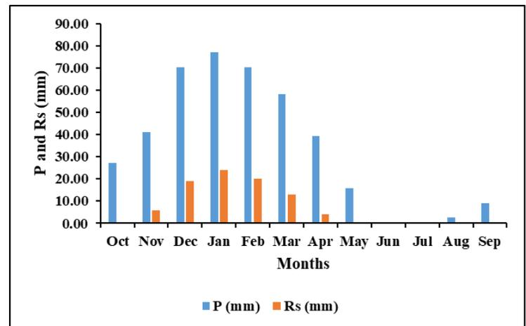
**Figure 8:** Relationship between mean monthly rainfall and runoff in (mm) which calculated by SCS method.
