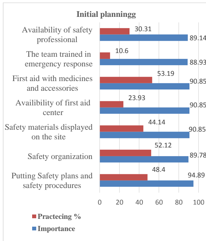
Figure 2: The percentage of average practice and average importance of the initial planning phase of safety management
