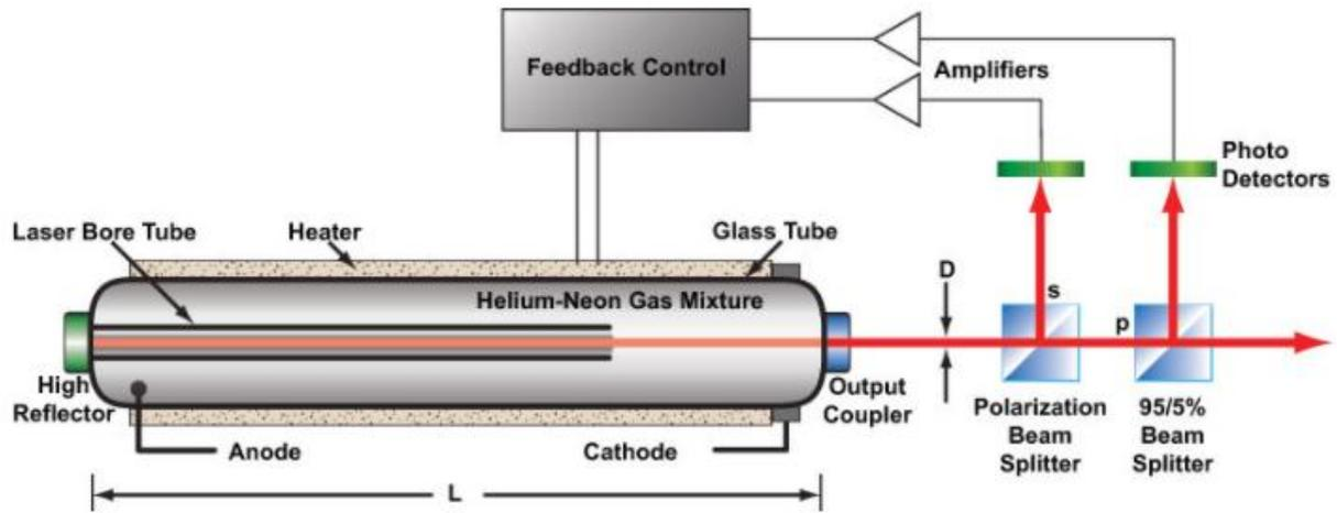
**Figure (1): Schematic diagram of a helium-neon laser consisting the optical cavity as comprised with the active medium and two parallel facing mirrors.**
