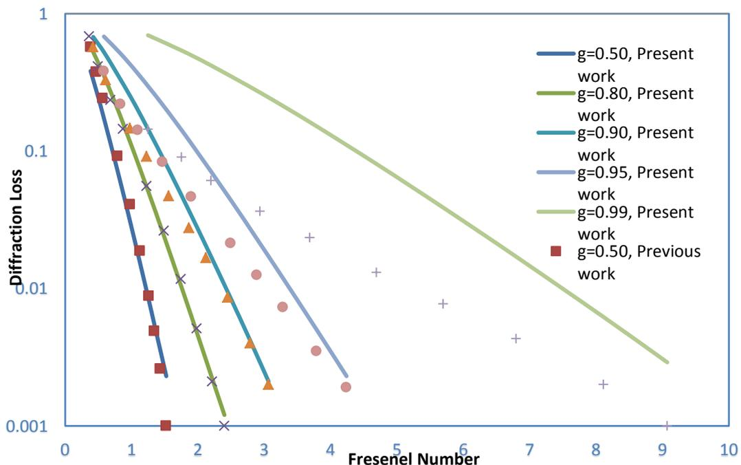
**Figure (3): Diffraction loss versus Fresnel number for the TEM<sub>01</sub> mode, for  $g=0.50$ ,  $g=0.80$ ,  $g=0.90$ ,  $g=0.95$  and  $g=0.99$  for both works.**
