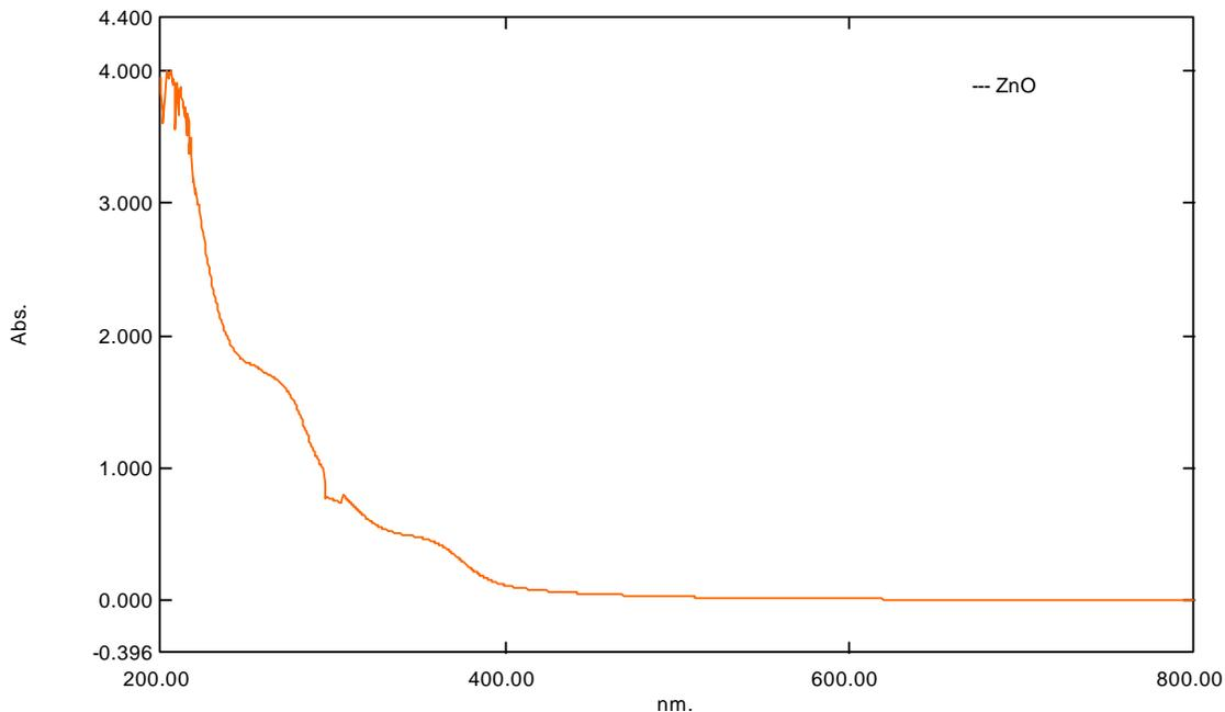
Figure 4: UV-vis spectrum of ZnONPs synthesized using River oak leaves
