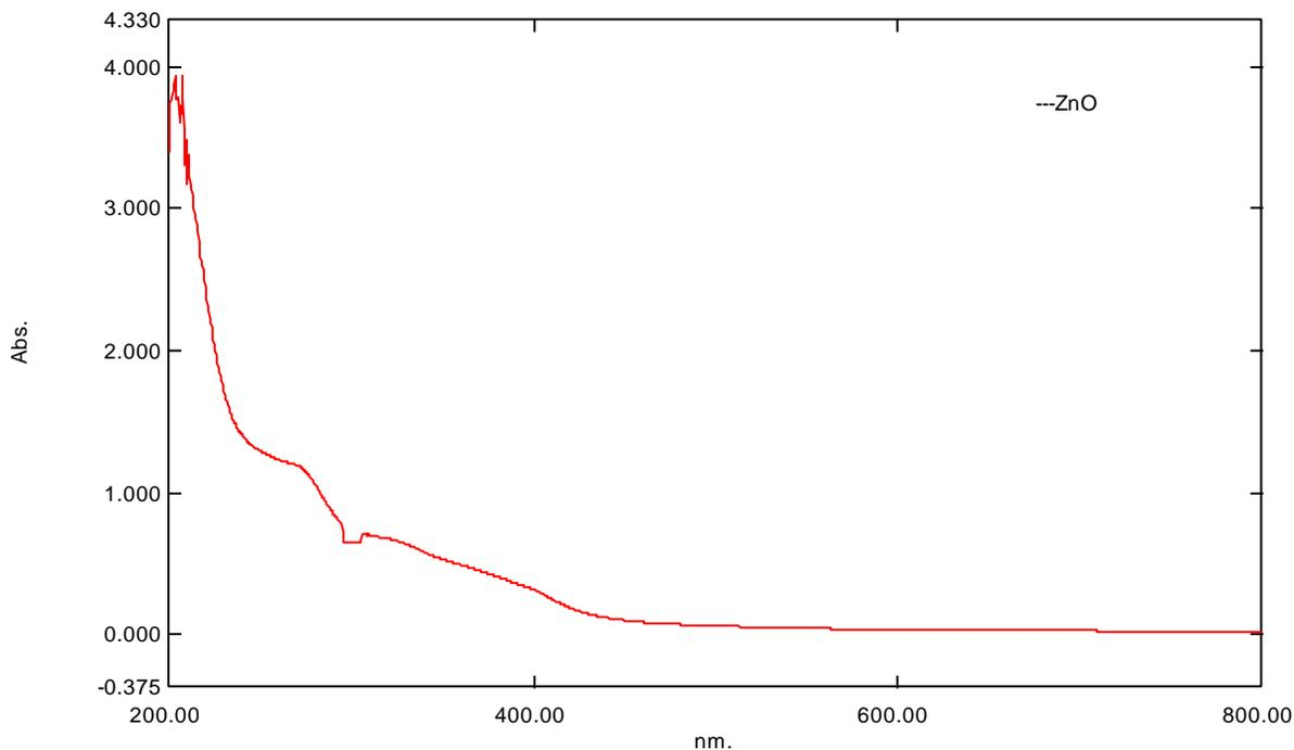
Figure 2: UV-vis spectrum of ZnONPs synthesized using Dill leaves
