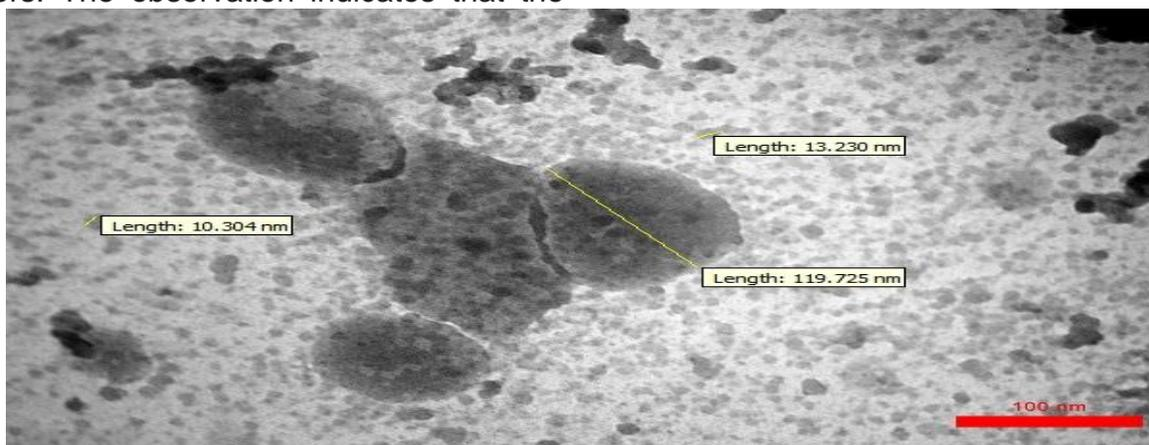
Figure 7: TEM image of green synthesized ZnO NPs from River oak plant
