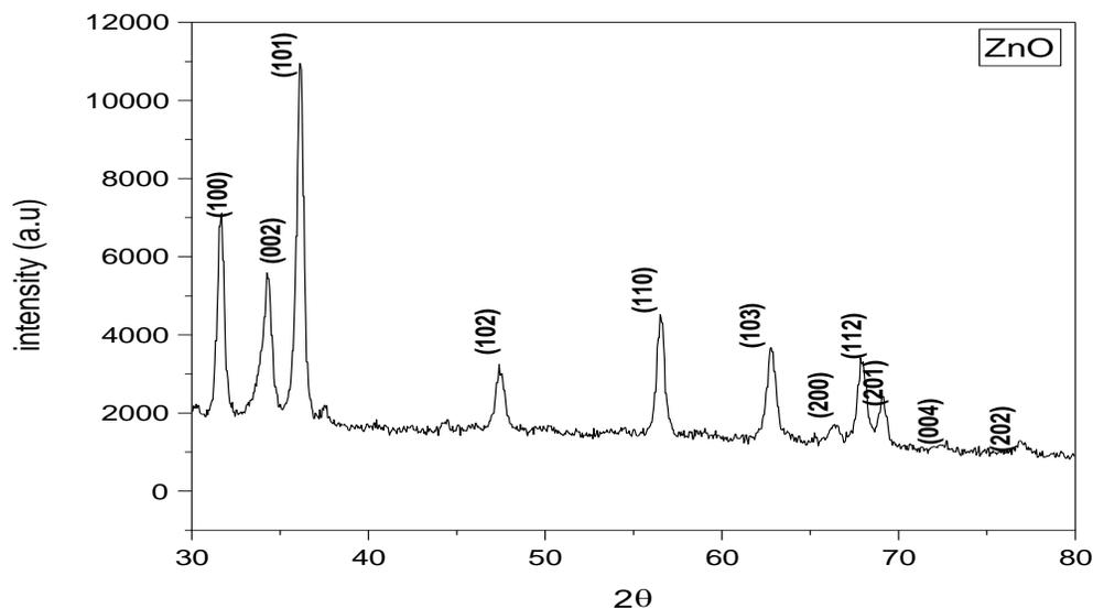
Figure 10: XRD pattern of ZnONPs synthesized using River oak plant
