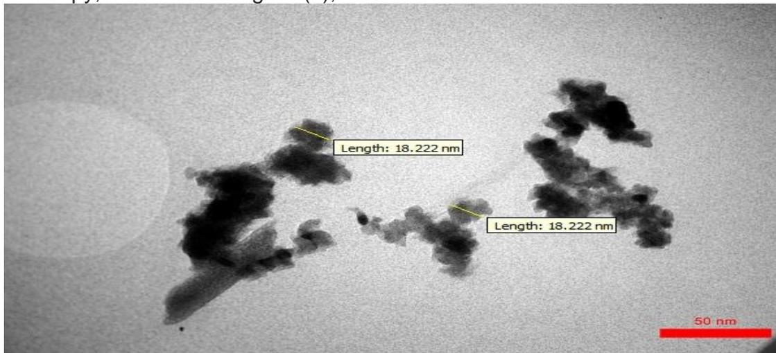
Figure 6: TEM image of green synthesized ZnO NPs from Eucalyptus plant
