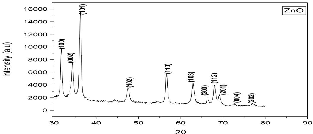
Figure 8: XRD pattern of ZnONPs synthesized using dill plant
