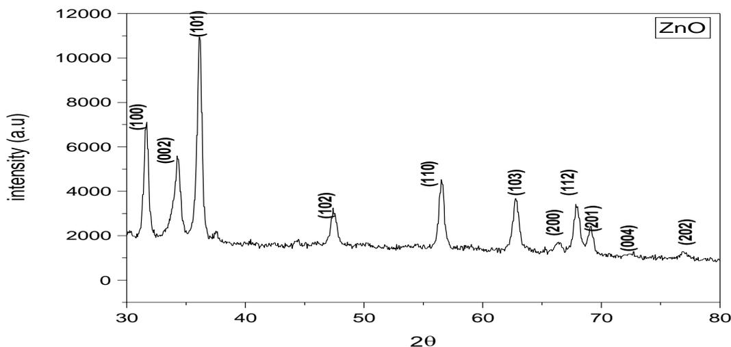
Figure 9: XRD pattern of ZnONPs synthesized using Eucalyptus plant
