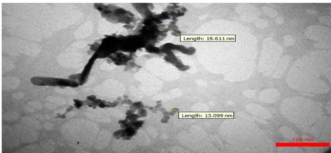
Figure 5: TEM image of green synthesized ZnO NPs from Dill plant
