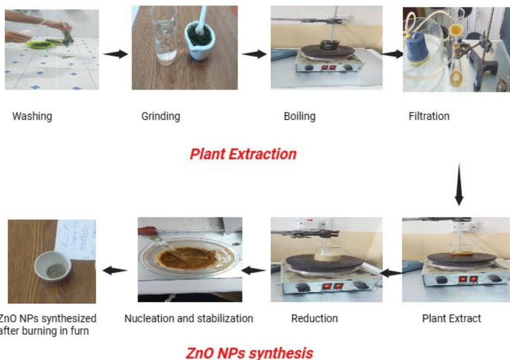
Figure 1: The process of Zinc Oxide nanoparticle synthesis
