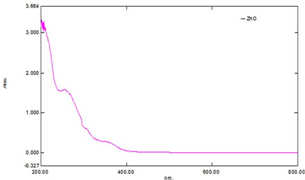
Figure 3: UV-vis spectrum of ZnONPs synthesized using Eucalyptus leaves
