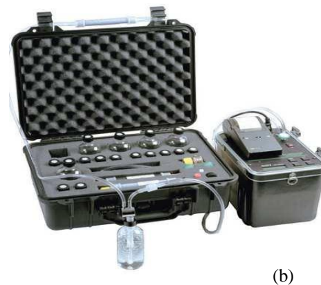
Fig. (3) General set-up RAD7 measurement technique, (a) schematic diagram for measuring radon in soil and building material samples, (b) RAD H 2 O accessory used to measure radon concentration in water.
