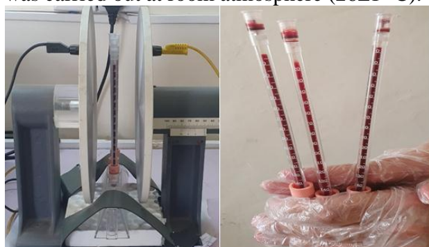
Figure 1: Electric field exposure setup and Westergren tubes.
