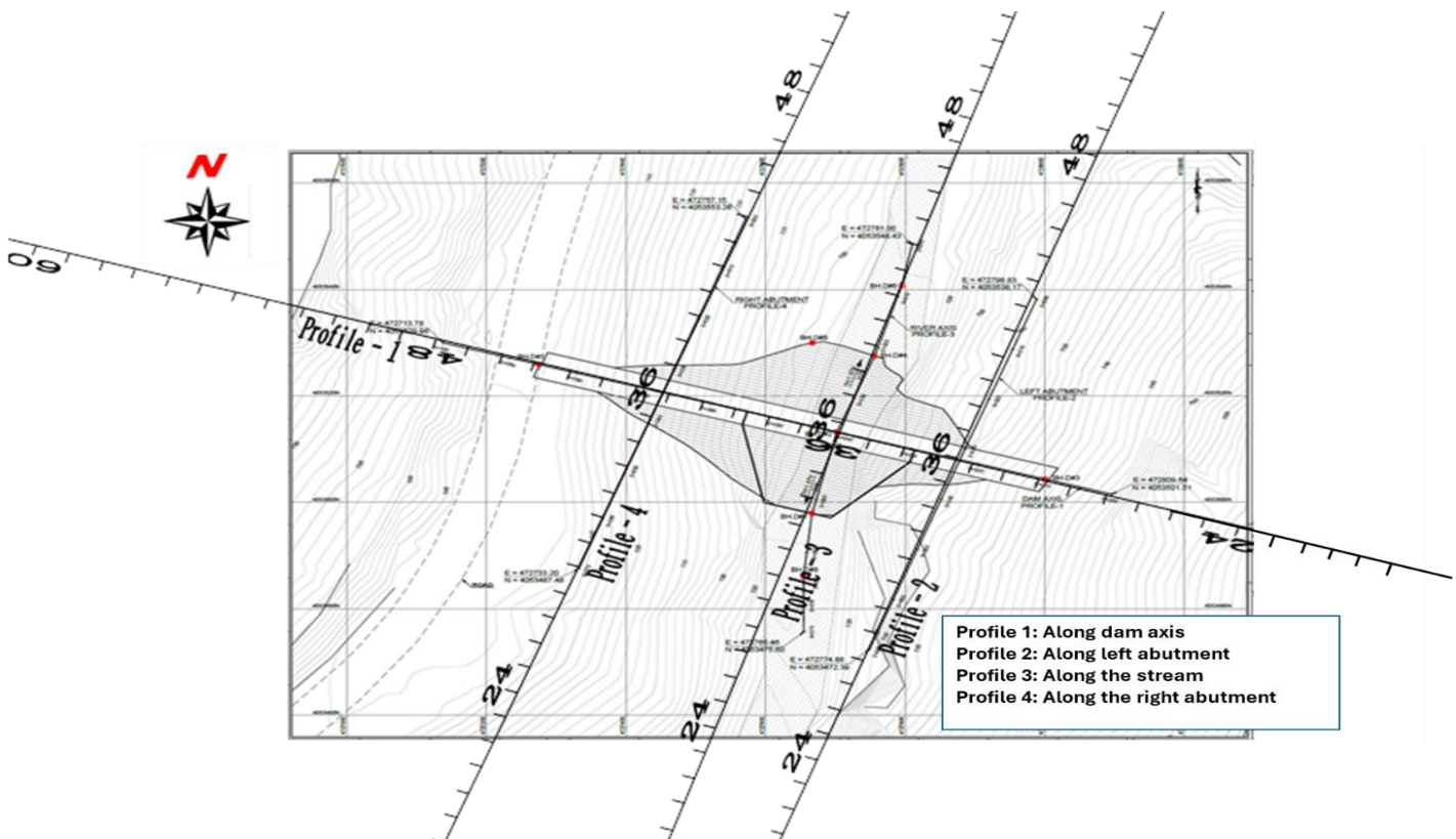
Fig.4: Display of profiles and electrode distribution
